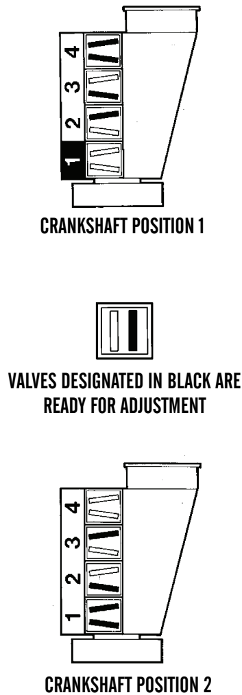
Figure 2. Crankshaft Positions 1 and 2.
